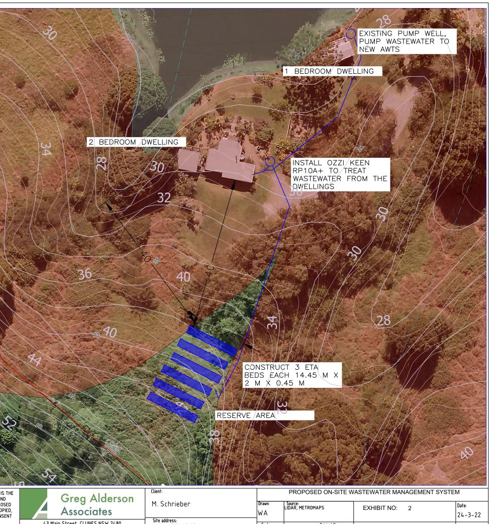
40 m Buffer to drainage lines
